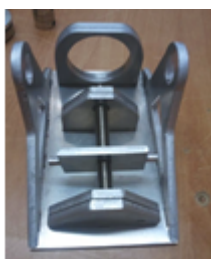
Fig. 1. Prototype of the ankle and ankle joint manufactured in lab Seletron SRL
